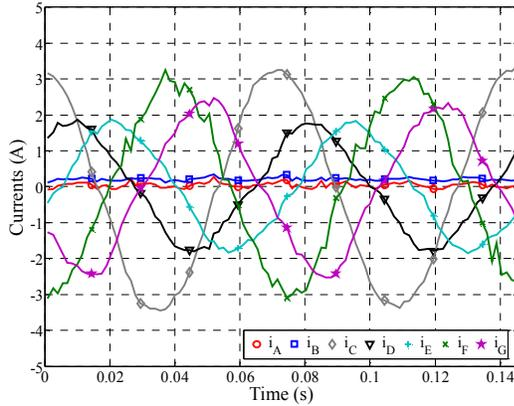
Fig. 11. Measured currents in fault operation without change of control
