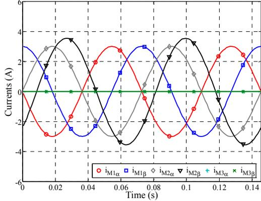
Fig. 6. Currents of the three fictitious machines in fault operation and improved control ( $I_{M1} = 3A$ )
