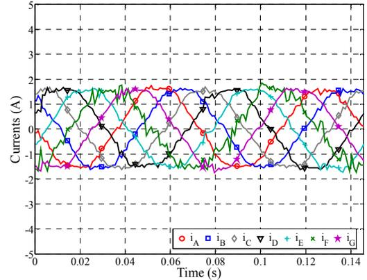
Fig. 8. Measured currents in normal operation
