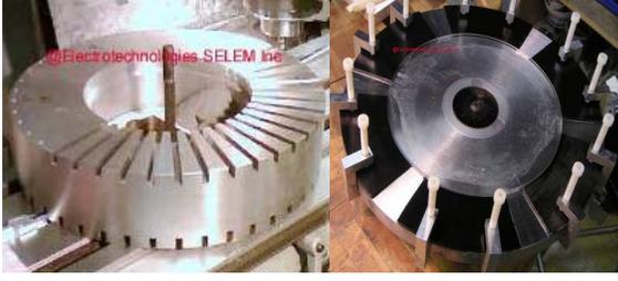
Fig. 3. Stator and rotor of the studied machine
