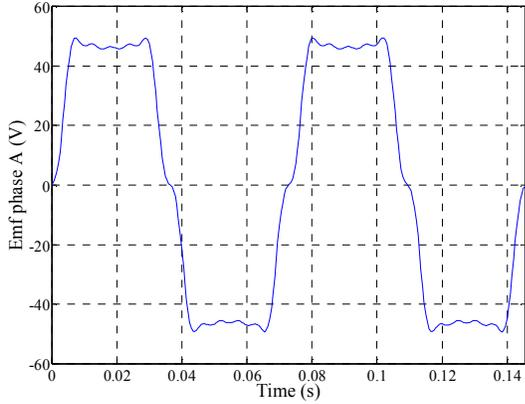
Fig. 4. Measured EMF of phase A at 275 rpm
