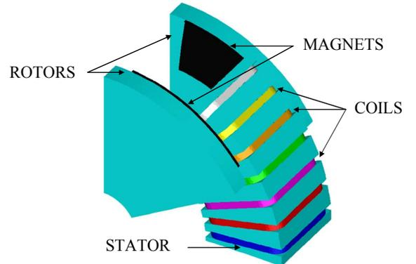
Fig. 2. One sixth of the axial flux seven-phase machine
