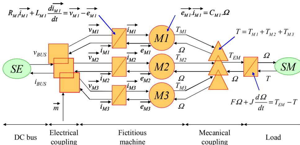
Fig. 1. Multi-Machine Energetic Macroscopic Representation of the seven-phase machine
